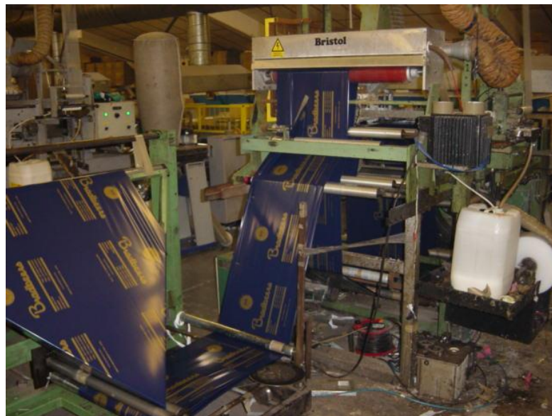
Figure 4: Side welding Machine (PPP, 2005-10).
